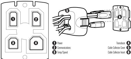
8. Line up the cable collector insert and cover, with the keying feature, then slide the cover into place on the insert.
